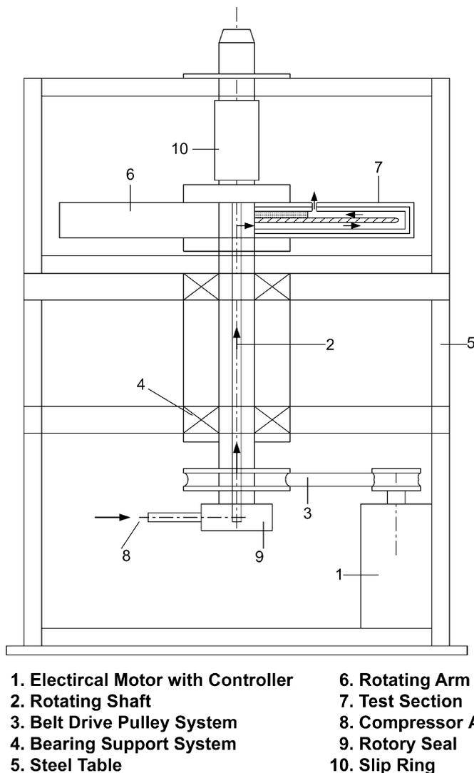
Fig. 1. Schematic view for the test rig.
